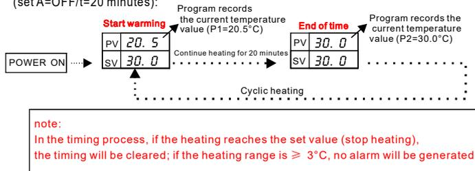
When the timing is over and the temperature rise is less than 3°C (P2-P1 < 3°C), the program considers this heating to be an "abnormal heating" behavior.
