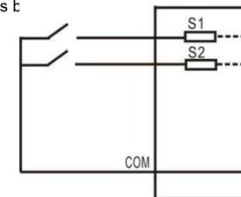
Generally, when external contact is ON, the linking status input channel on CHD9001 LCD will be ON. When external contact is OFF, the linking status input channel on CHD9001 LCD will be OFF.
